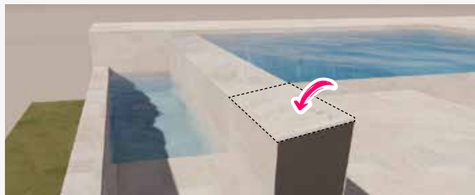
Infinity Pool Channel wall 50 cm wide.
